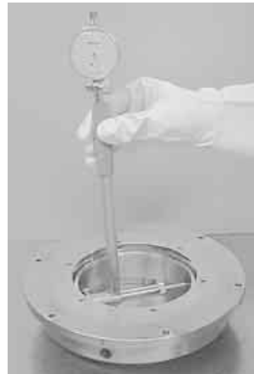
Fig. 1.10 Zero Setting of Cylinder Gauge
